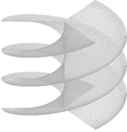
FIG. 1. Schematic representation of the wave front for a typical l = 3 optical vortex, over the span of three wavelengths. The interval between successive wave fronts is one wavelength.
